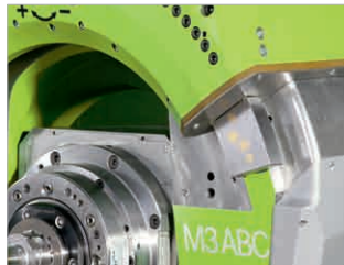
The key to the innovation is the specially developed, very rigid and precise curved guideways of the B-axis.
