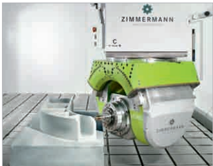
3-axis simultaneous milling without pole situation and still large swivel ranges – this is only possible with the M3 ABC.
