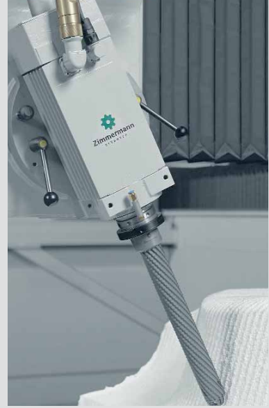
Milling head on FZ 15 3+1 axes
