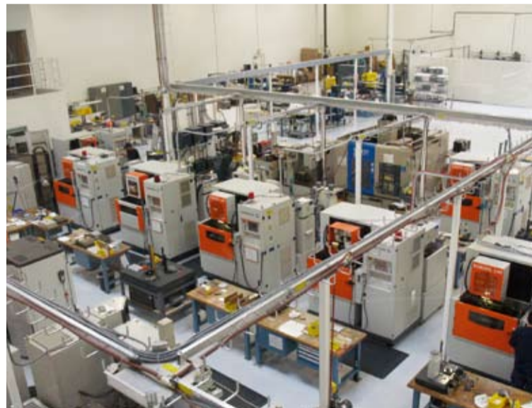
← The EDM machines from GF AgieCharmilles meet Classic's high standard for electro-discharge machining.
