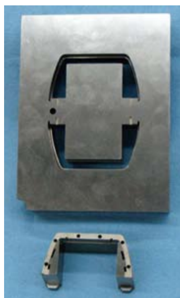
↑ Mold inserts for an 8-fold injection mould for the production of partitions for light bars which are mounted on security and ambulance service vehicles.
