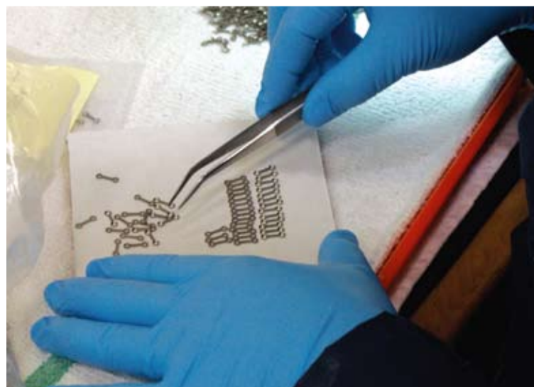
← EDM wire-cut parts are subjected to a visual inspection.
